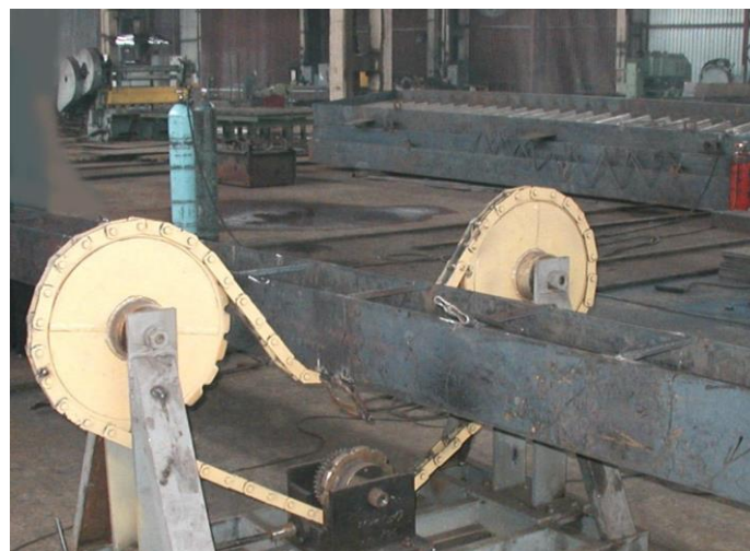
Figure 10 – Positioning of a Welded I-Beam Profile with a Corrugated Web on a Rotator for Welding Flange Joints with Unequal Fillets.
