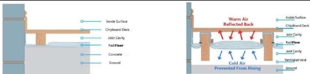
Figure 8 - Example of a suspended timber floors insulation with reflective multi-foil insulation
