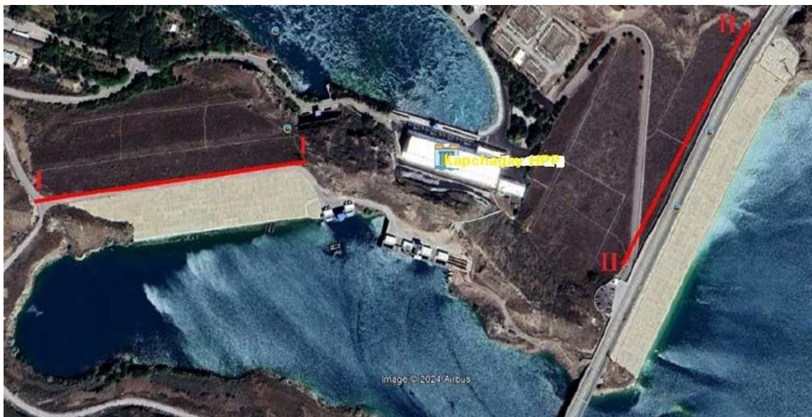
Figure 3 - Alignment lines to control horizontal displacement (marked in red).
