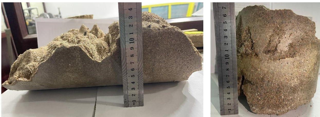
Figure 3 – Example of sand consolidation with two-component resin in laboratory conditions (author's material).
