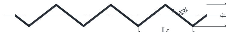
The corrugation thickness t_w is 1.9 mm The corrugation wavelength L_r is 350 mm; The corrugation height f_r is 54 mm.
