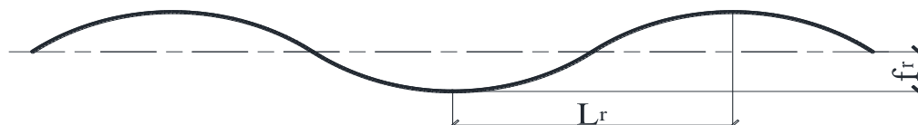
Figure 4 — Beams with cross-corrugated web and wavy-shaped corrugations: L_r – is the length of the corrugation half-wave; f_r – is the height of the corrugation half-wave (the authors' material).
