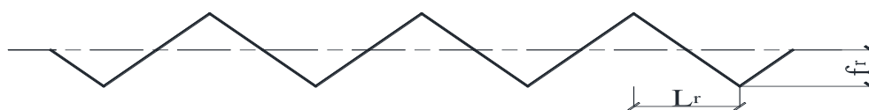
Figure 1 – Beams with cross-corrugated web and triangular-shaped corrugations: L_r – is the length of the corrugation half-wave; f_r – is the height of the corrugation half-wave (the authors' material).
