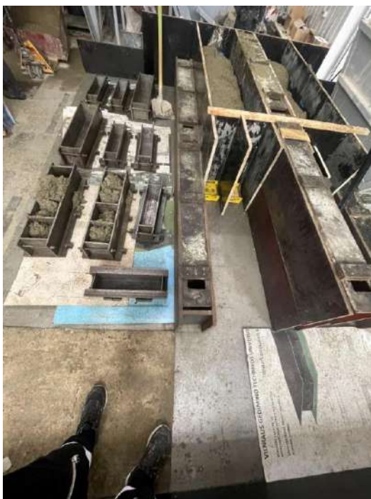
Figure 5 – Cube, prisms molding form (author's materials)
