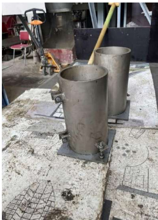
Figure 4 – Cylinder molding form (author's materials)
