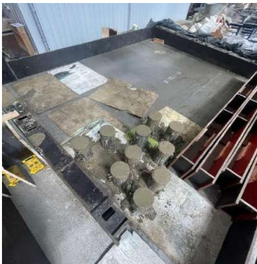
Figure 6 – Preparation of cylinder-shaped specimens (author's materials)
