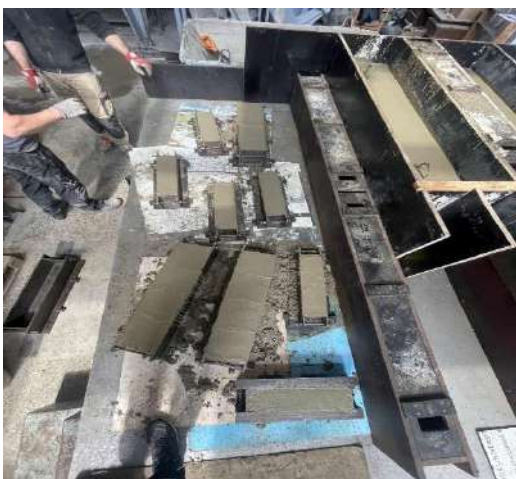
Figure 8 – Preparation of cube-shaped, prism-shaped specimens (author's materials)
