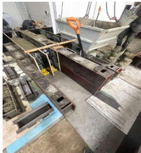
Figure 7 –Preparation of cube-shaped, prism-shaped specimens, cylinder-shaped specimens (author's materials)
