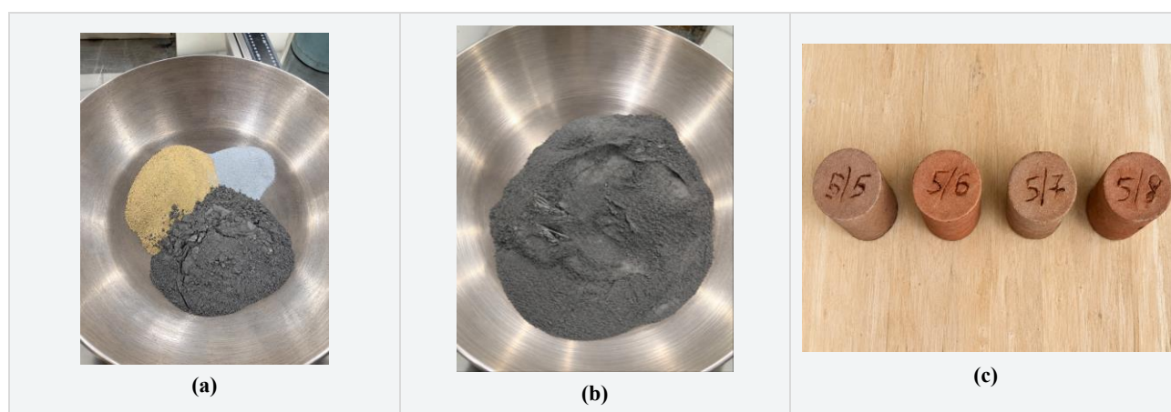
Figure 6 – Principal laboratory stages: (a) raw-material components before mixing; (b) prepared ceramic body after mixing; (c) cylindrical specimens after firing [Author's material]
