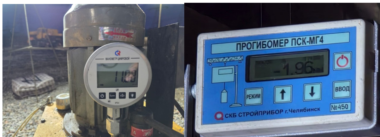
Figure 5 - Instruments used during static load testing [Authors' material]
