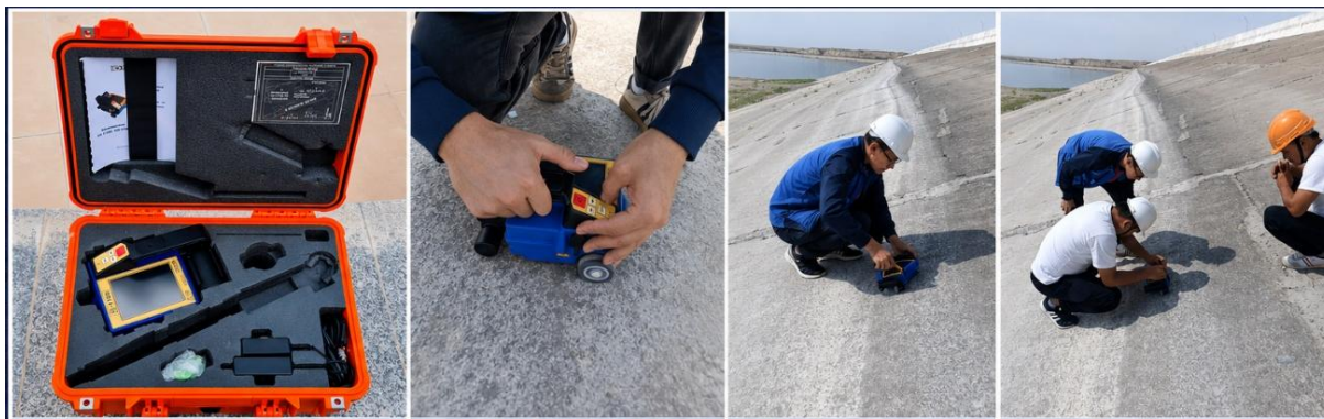
Figure 3 - Field application of the CK-1700 3D ultrasonic tomography system during inspection of concrete structures at the Tasotkel Reservoir emergency spillway (authors' material)
