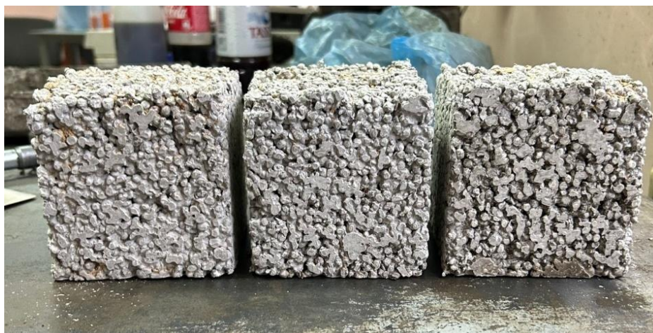
Figure 1 – Polystyrene concrete samples with a water-binding ratio (W/B) = 0,45 (author's material)
