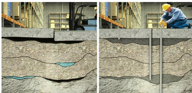
Figure 5 - Soil reinforcement by injection method (catalogue SK Stroiz, 2024)
