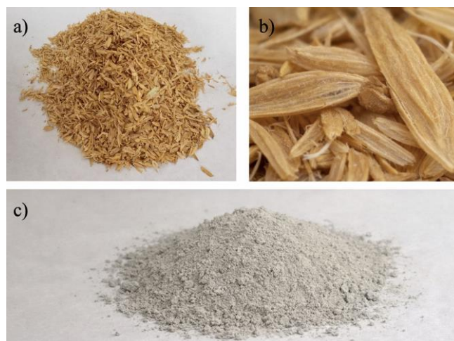
Figure 1 – Materials used in the study: (a) raw rice husk (general view); (b) raw rice husk particles (magnified view); (c) portland cement [author’s material].
