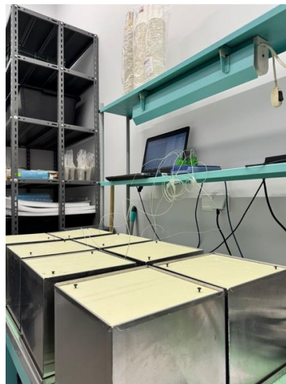
Figure 2 – Experimental setup used to monitor the evolution of temperature during cement hydration (author’s material)
