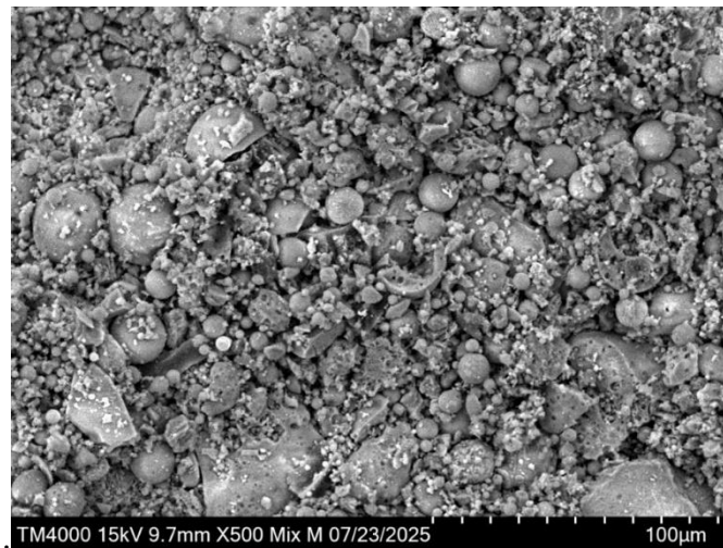
Figure 2 – Microstructure of unactivated fly ash (SEM, ×500) (author’s material)
