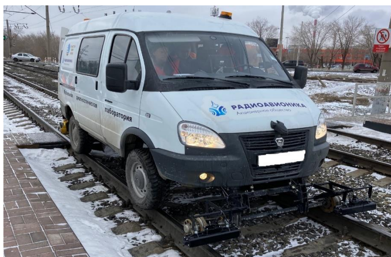
Figure 1 – General view of the mobile diagnostic laboratory on the road–rail platform [Authors' material]
