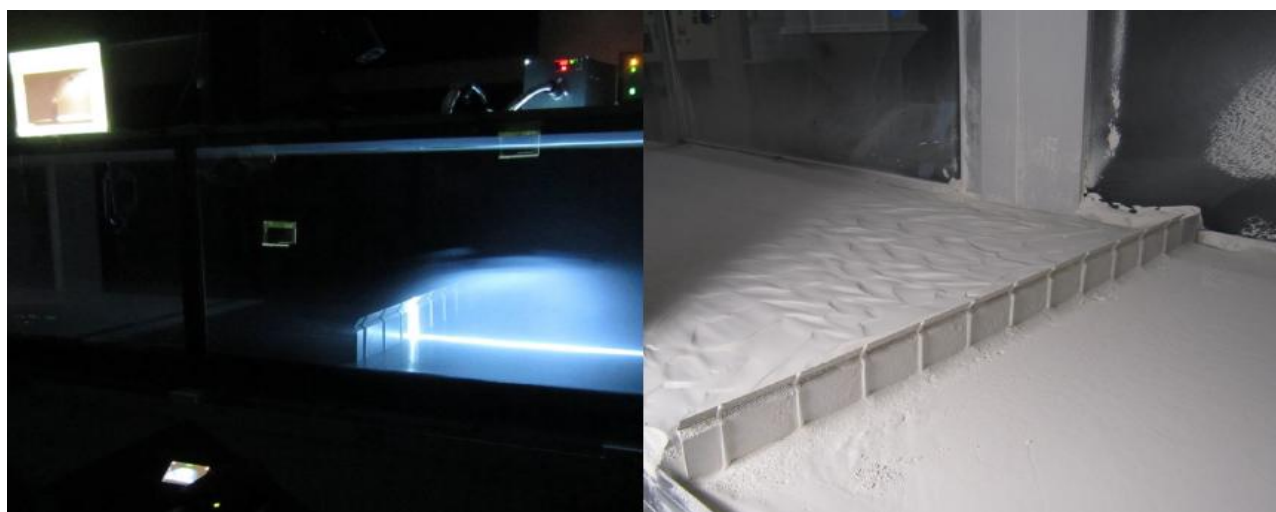
Figure 2 – Models of snow protection fences in a wind tunnel [7]
