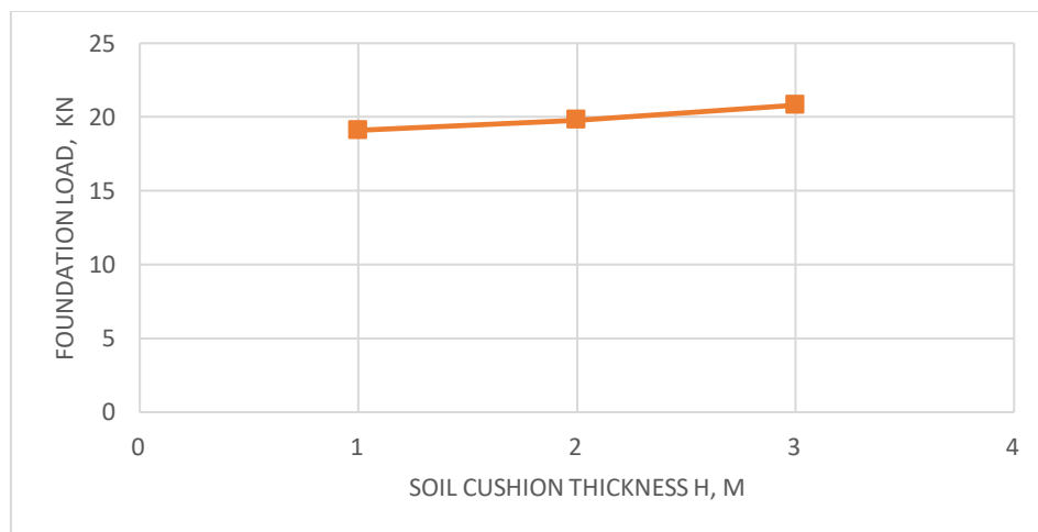
Figure 27 – Relationship between foundation load and soil cushion thickness ) (author's material)
