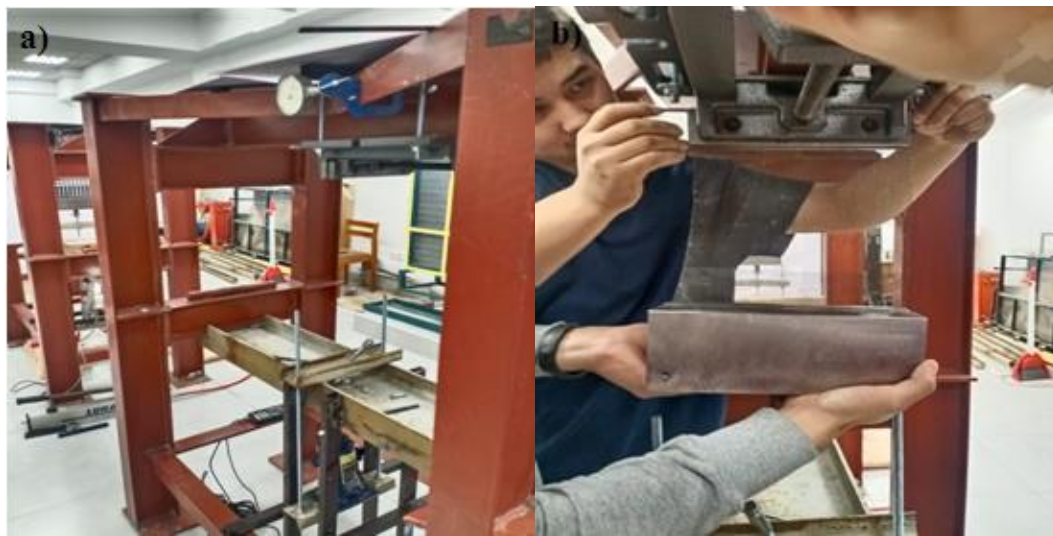
Figure 2 – Tensile testing machine of the geotechnical laboratory (a) and the process of conducting a tensile test of a geogrid sample (b) (author's materials)
