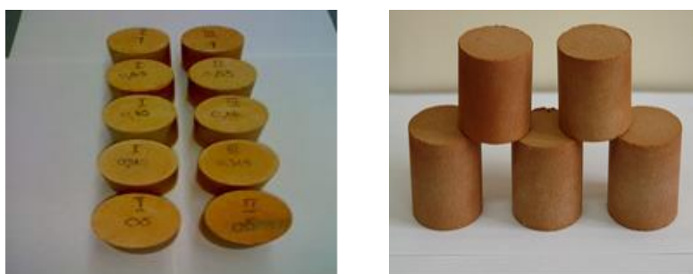
Figure 7 – Laboratory heat-treated cylindrical samples at a temperature of 1000 °C (authors material)
