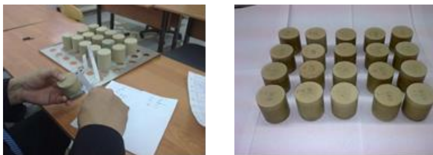
Figure 6 – Laboratory green cylindrical samples (authors material)
