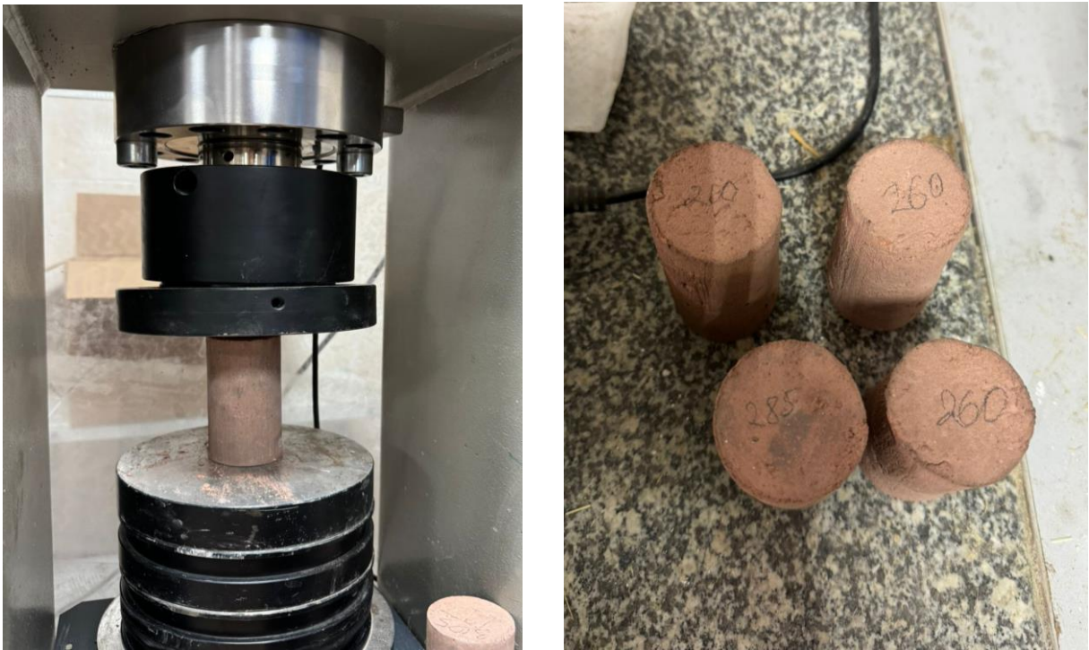
Figure 5 – ceramic material based on wood waste and testing its compressive strength (author’s material)
