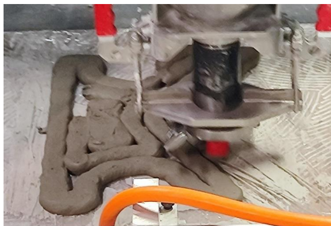
Figure 7 – Photofixation of the fracture process (loss of shape stability with displacement of the printed layers) of a sample printed on a 3D printer
