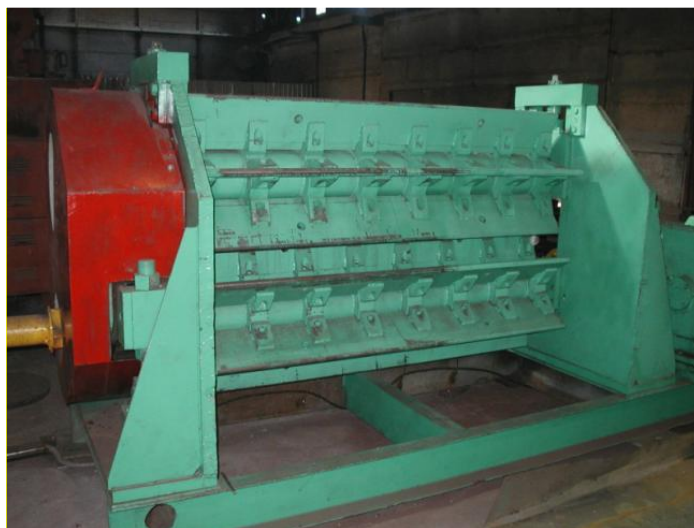
Figure 6 – Rotary Machine for Continuous Corrugation of Steel Sheets.
