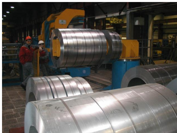
Figure 8 – Universal Steel Coils for I-Beam Webs.
