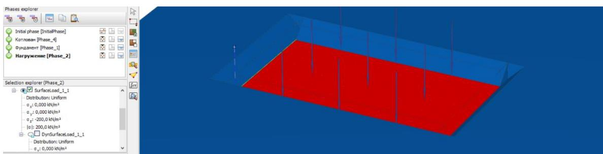
Figure 6 – Average pressure of 20.0 t/m<sup>2</sup>.
