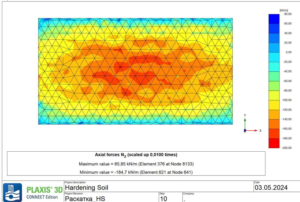
Figure 11 – Foundation. Axial force N, Hardening Soil model (max 184.7 kN/m).
