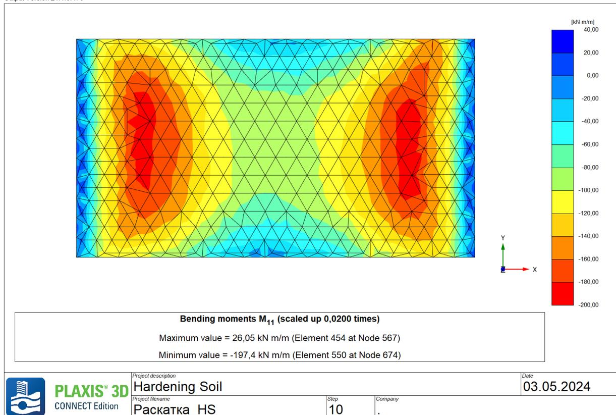
Figure 12 – Foundation. Bending moment M, Hardening Soil model (max 197.4 kN·m/m).
