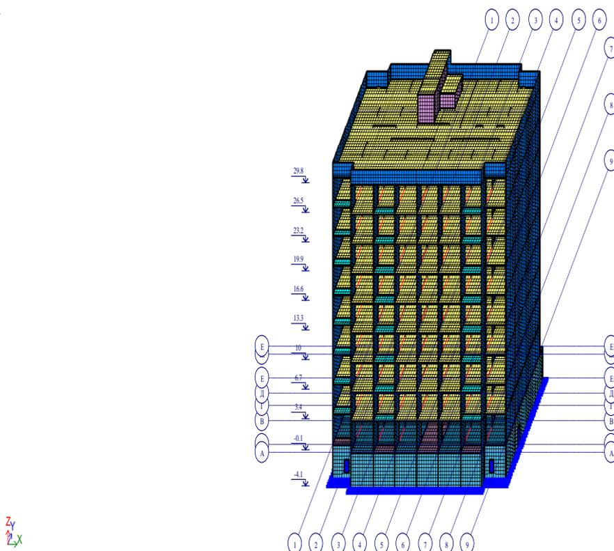
Figure 2 – Structural Scheme of the Residential Building.
