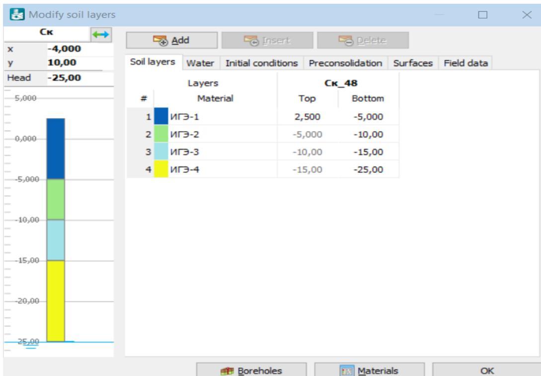
Figure 3 – Geological model in PLAXIS software.
