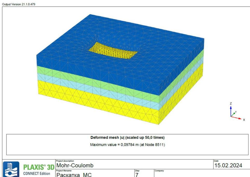
Figure 7 – Deformation pattern (Mohr-Coulomb model).
