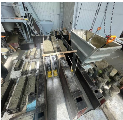
Figure 9 – General view of the molding forms with cast concrete specimens (author's materials)
