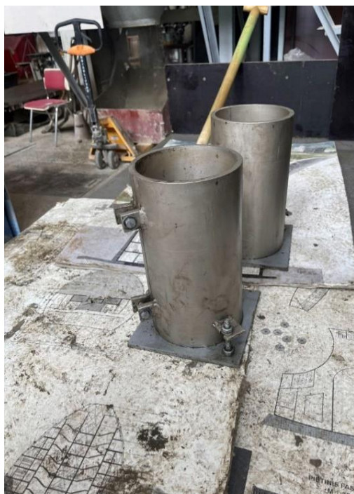
Figure 4 – Cylinder molding form (author's materials)
