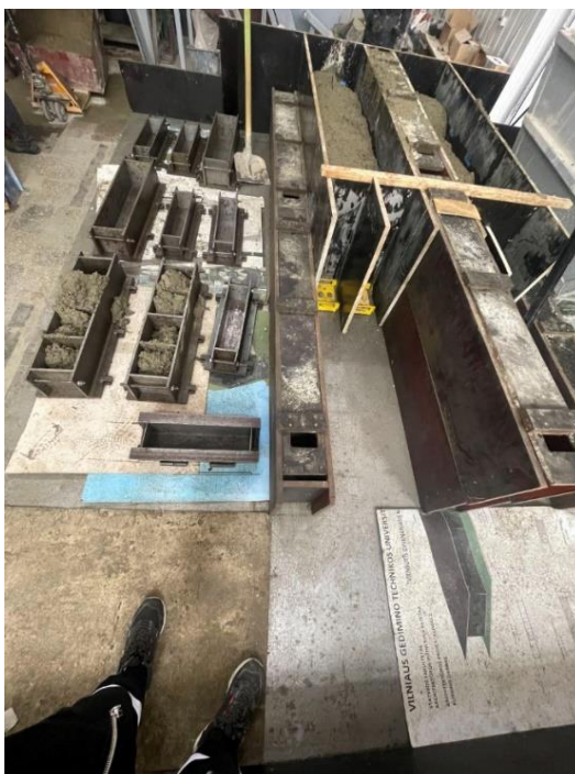
Figure 5 – Cube, prisms molding form (author's materials)
