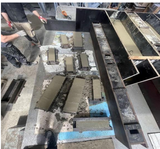
Figure 8 – Preparation of cube-shaped, prism-shaped specimens (author's materials)
