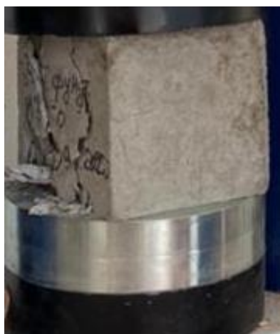
Figure 11 – Strength tests on the specialized press machine in the laboratory of Vilnius Gediminas Technical University (VILNIUS TECH) (author's materials)
