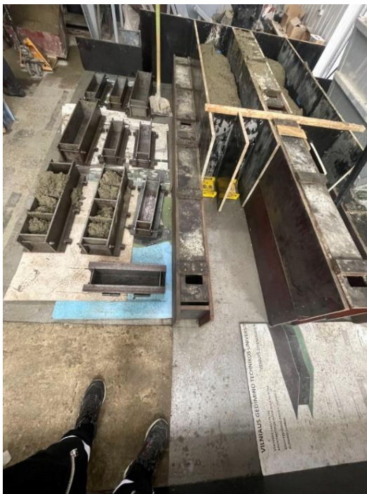
Figure 5 – Cube, prisms molding form (author's materials)
