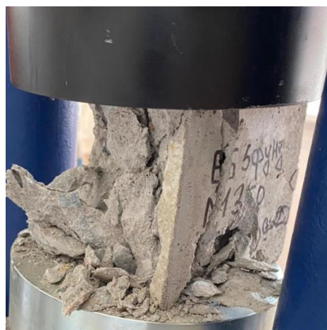
Figure 12 – Strength tests conducted on a specialized press machine in the laboratory of Vilnius Gediminas Technical University (VILNIUS TECH) (author's materials)
