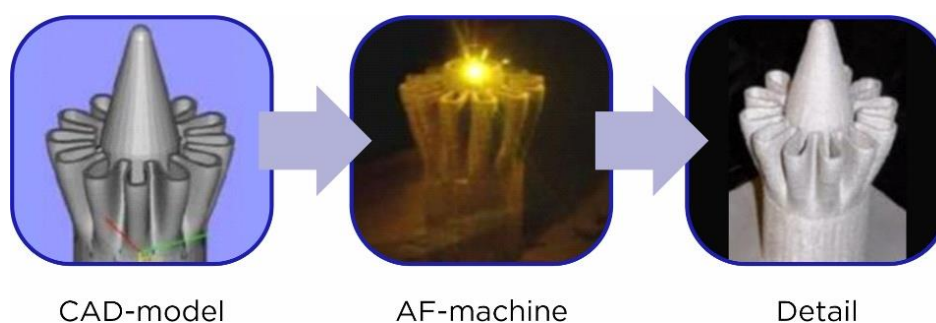
Figure 1 – General diagram of the process of creating a 3D model
